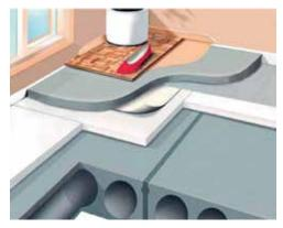
The standard thicknesses of the BEWI Step boards are 20 mm and 30 mm. They are suitable for floor structures with standard loading of less than 5 kN/m $^2$  – Thus, BEWI Step is also an excellent choice for aisle spaces with loads higher than normal floor structure.
