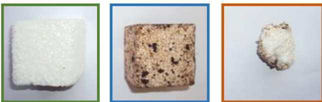
Figure 3: Samples for composting (left: start, middle: after cold composting, right: after industrial composting)
