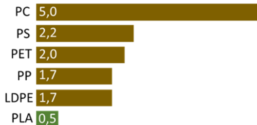
Figure 2: Carbon footprint of PLA compared to other fossil based polymers (Kg CO 2 eq per Kg polymer)
